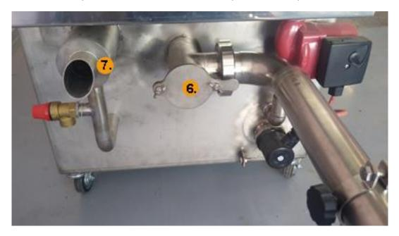
Both heating elements are pre-set to specific temperatures. The tank bottom is set to 34-37°C, and the radiator is set to 74-78°C. The temperature controllers maintain the temperatures of the tank and the radiator within these specified ranges. The heating mat's temperature controller activates if the tank temperature drops below 30°C and deactivates when it rises to around 32°C. The heating indicator
